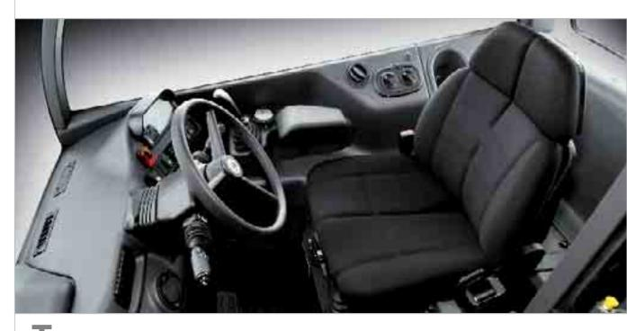
he standard, continuously adjustable, tilting steering column grants a full range of operator adjustments to provide his most suitable driving position.
